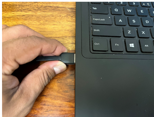
Figure 5: Type-A end of micro USB cable connected to laptop USB port
