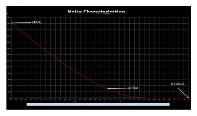
So how will this be used? That's tricky...If you consider below image, where victim output which is supposed to be at logic '0', suddenly sees an c in its voltage level due to nearby aggressor attacking it. In such cases, you just need to keep on measuring current of respective vin and Vout.
