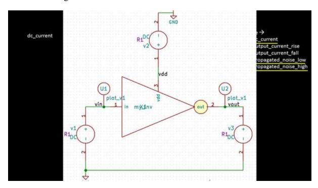
This needs a 2-dimensional DC sweep analysis, where input voltage is swept for a constant output voltage, and static current is measured at output node 'Vout' for each swept input voltage point. Next, we sweep output voltage by a unit, and again, the input voltage is swept for that new output voltage, while we dump dc\_current scalar values for each combination of input and output voltage. Below is how it looks like:
