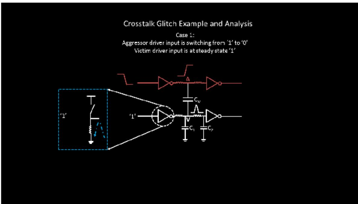
In the above case, the inverter (NMOS specifically) could discharge the glitch completely, thus making this one as a 'safe glitch'. And just now, I introduced you to 2 new things .... 1) a way to reduce glitch, and 2) the term 'safe glitch'.
