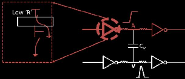
In this one, I have represented resistance by a box. Wider the box, least is the resistance, more area available for current to flow from supply to output load, and hence faster it will charge the output load.
