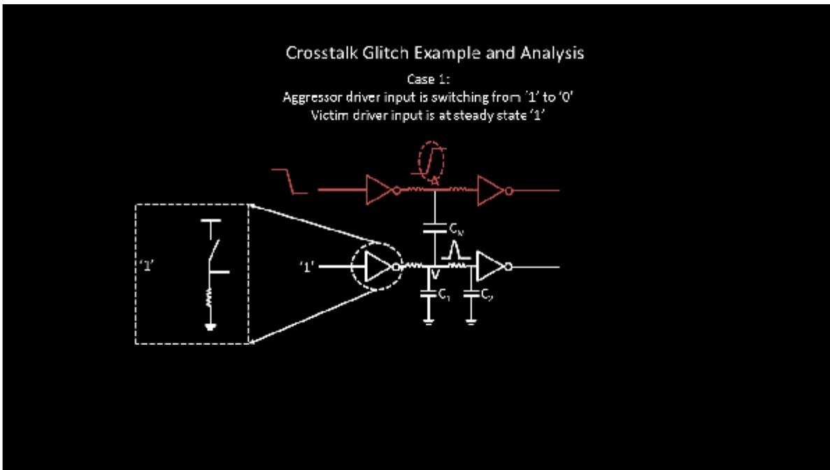
In a situation like this, a glitch becomes an issue, if the inverter is not able to completely discharge the extra 'charge' deposited by the aggressor.
