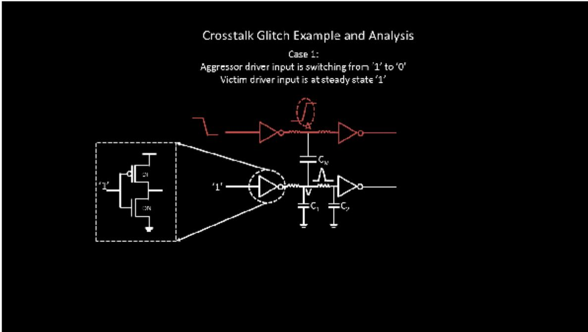
The off PMOS can be replaced by an open switch and on NMOS can be replaced by a resistance like below
