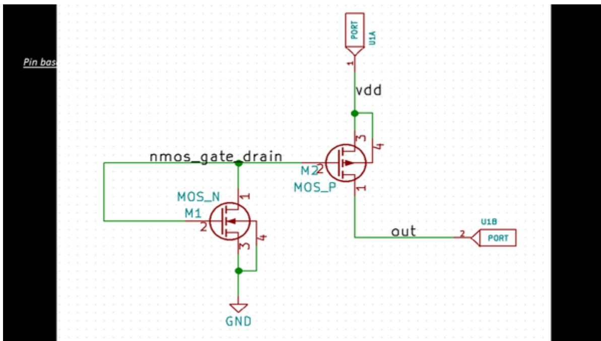
You see the connections for NMOS transistor ‘M1’. It forms a strong reverse biased diode whose output goes to PMOS transistor ‘M2’. Now here’s the puzzling waveform at the output port
