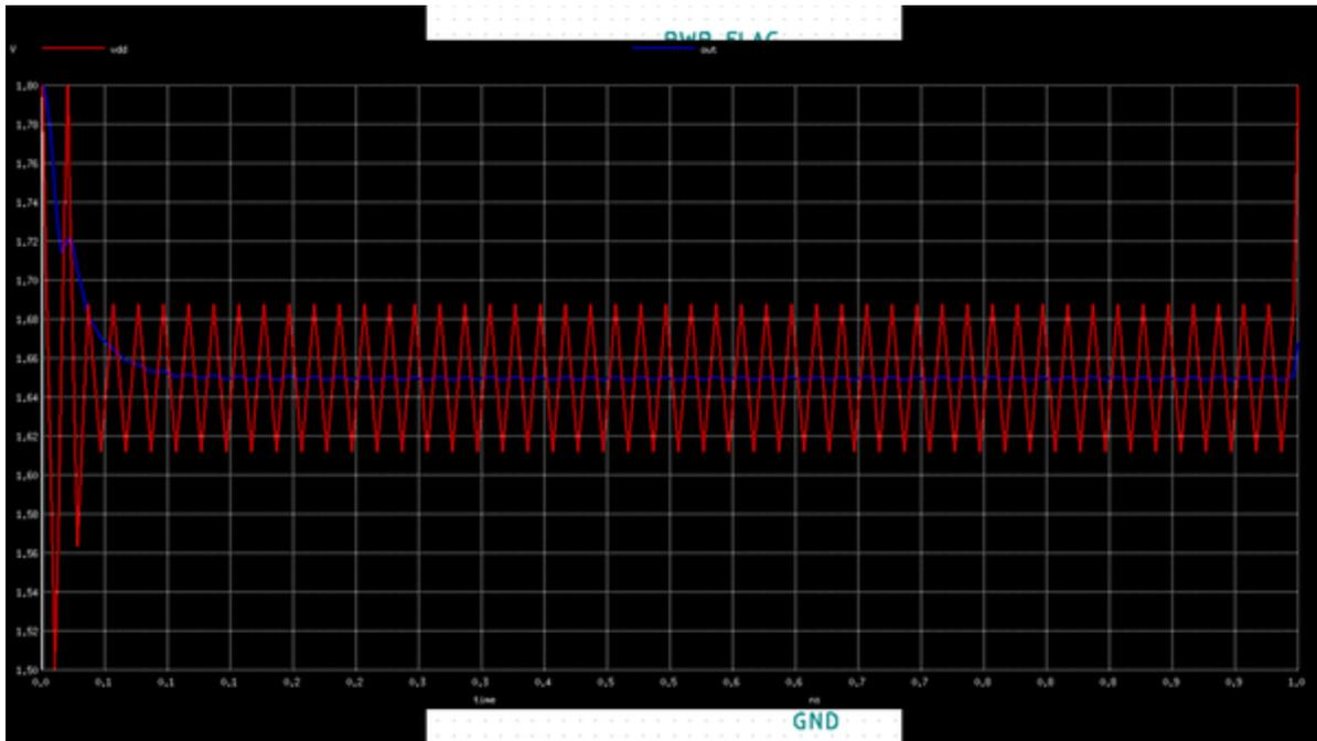
The 'red' waveform at 1.8v is the power supply distortion, famously called as voltage droop. And the 'blue' waveform is what you see at the output of tie-high cell. Looking closely at the VDD and tie-hi output, it appears to be something like below:
