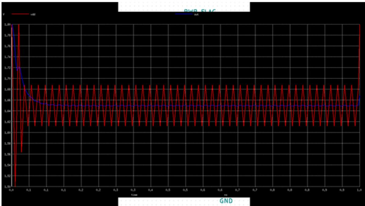
Now this VDD distortion is on the range of 70mV which is enough to damage 'gate oxide'. But the variation at the output of tie-hi cell is minimal and so it's the tie-hi that protects your gate oxide and hence the entire logic cell from being damaged.
