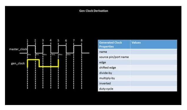
This is a classic example of how 'edge' and 'shifted edge' option of generated clock can be used in conjunction. Let's the first fall edge is in middle of 2ns and 4ns i.e. at 3ns
