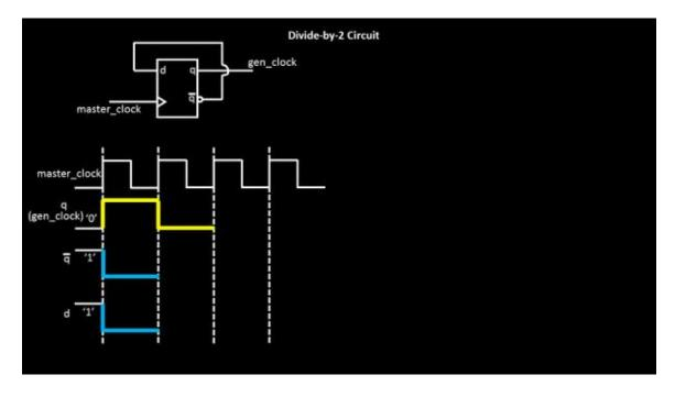
If you start with master clock of say ins period, the output is expected of 2ns period (frequency divide-by-2). So at the first rising edge of clock (assuming the initial state of circuit is 'q' = 0 and 'd' = 1), the data at 'd' pin will be propagated at 'q' output (since it's a rise-edge triggered flop), and 'q' becomes 'i', 'q\_bar' becomes 'o', and 'd' is at 'o'
