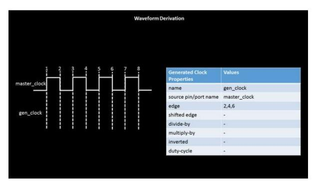
So, the above table, says, the first rise edge of the generated clock arrives at  $2^{nd}$  edge of master clock (remember, it doesn't matter whether  $2^{nd}$  edge of master clock is a rise or fall), the first fall edge of generated clock arrives at  $4^{th}$  edge of master clock and second rise edge comes at  $6^{th}$  edge of master clock and below is how your generated clock will look like
