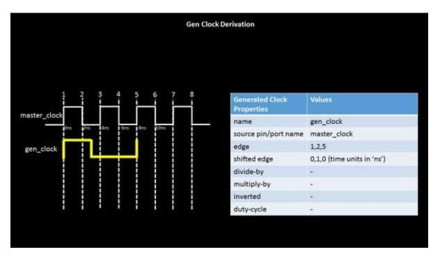
(...sentence continued from above image) the same gen\_clock' can be defined using just the edges, and removing options of the table. And below is how the generated clock definition will look like for gen\_clock'
